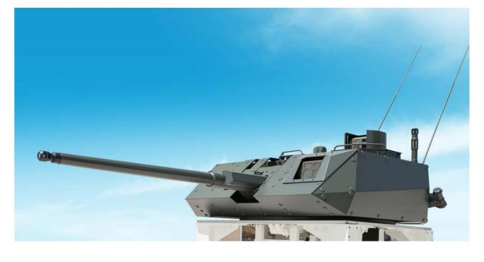
The TEBER-30 Two-Man Turret, is a medium caliber turret that can be fitted to wheeled and tracked armoured vehicles and is offered in two configurations. In the conventional two-man configuration, the commander and the gunner are positioned in the turret basket.
